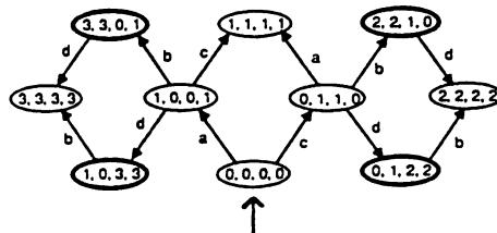
**Figure 11** Automate asynchrone reconnaissant  $\{[ab], [ad], [cb], [cd]\}$
